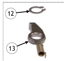
DETAIL, PAWL MOUNTING DIRECTION.
